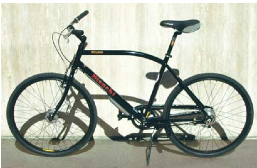
FREEWHEELING: No shift levers are on the handlebars of this Bianchi Milano bicycle. Instead an automatic transmission system senses acceleration and does all the gearshifting.
